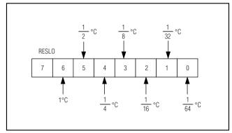
Figure 1. Temperature Measured in 1/64°C Steps
