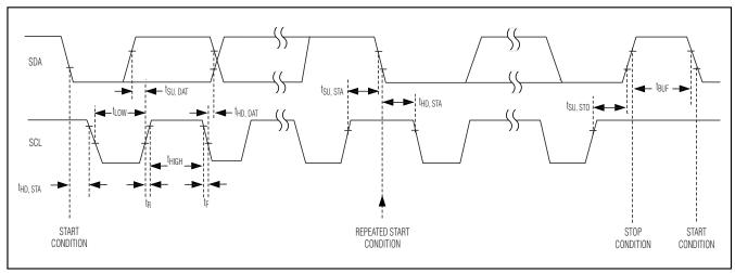
Figure 5. 2-Wire Serial-Interface Timing Details
