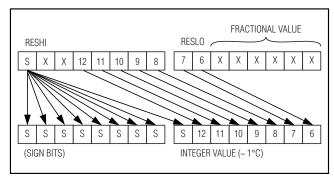
Figure 3. Alternate Temperature Representation
